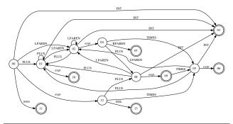
**Figure 2.** An LR(1) automaton for the grammar of Figure 1.
